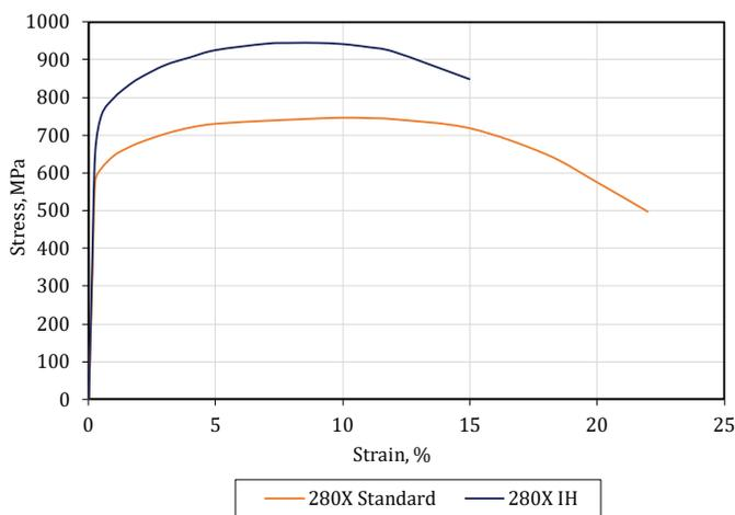
Fig 1: Stress-strain curves in tension for full section hard-chrome plated bar comparing hardened and non-hardened execution (280X-grade, diameter 30 mm). Depth of hardening for the IH-bar is 1.6 mm.
