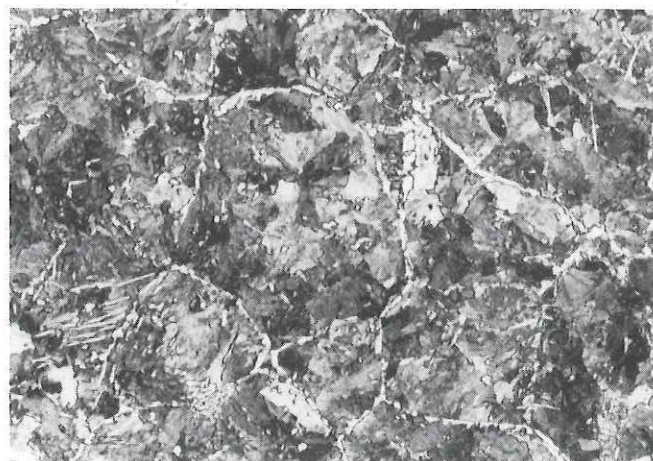
Fig 3 Steel 7, air cooled from 1150°C, 200 x.
