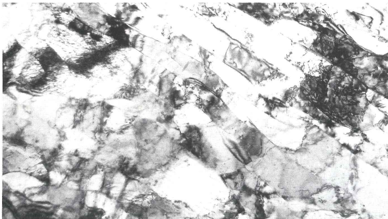
Fig. 1. Transmission electron micrograph of the ferrite matrix of cold rolled and annealed grade SKF 280. The dislocations have largely rearranged themselves into subgrain boundaries, with low dislocation densities within the subgrains. Subgrain size: 0.2–0.5 \mu\text{m} (8–20 \mu\text{in} ).
