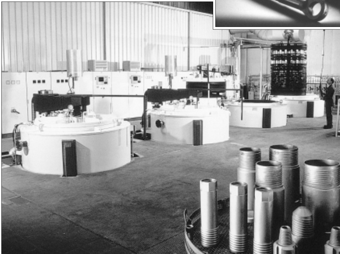
Figure 16. Plasma Ionitox furnace line at Bodycote's workshop in Ludenschied, Germany.
