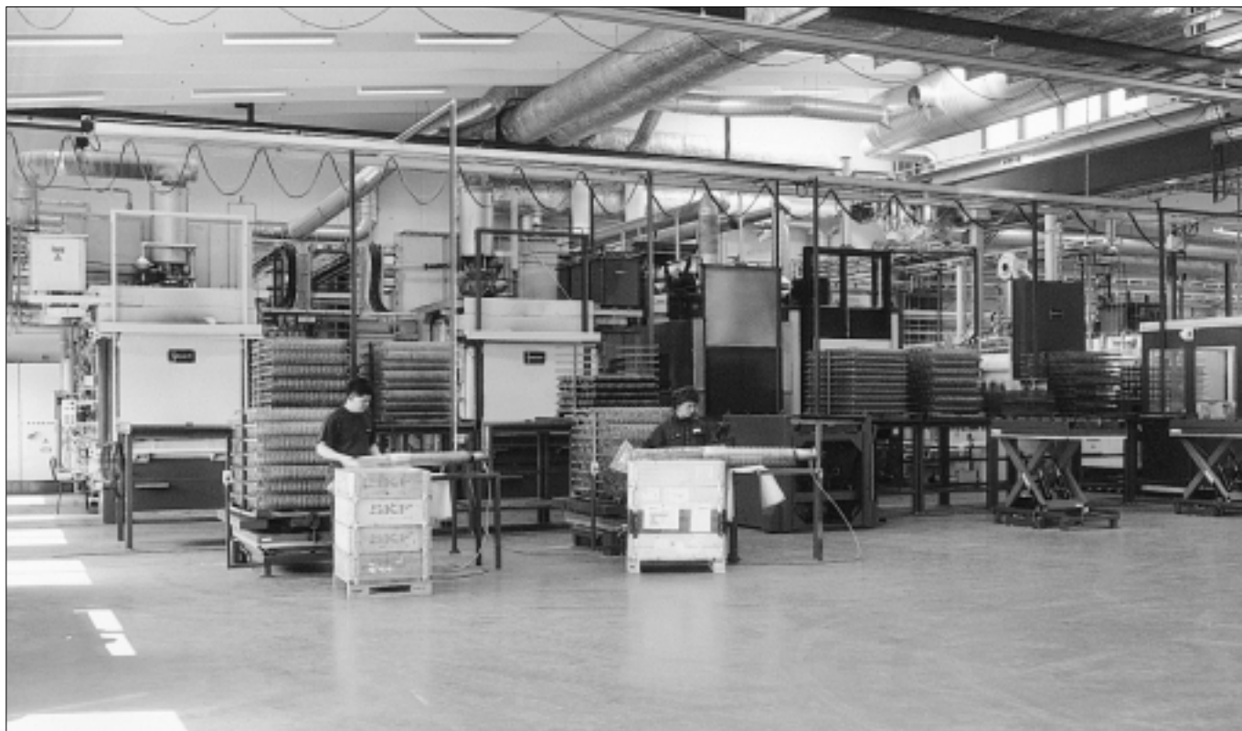
Figure 14. Furnace line used for the Colournite process at Bodycote Brukens workshop in Gothenburg, Sweden.
